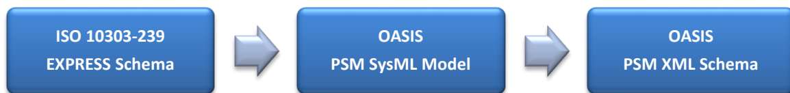
Figure 44: ISO STEP AP 239 to OASIS PSM information model transformation
